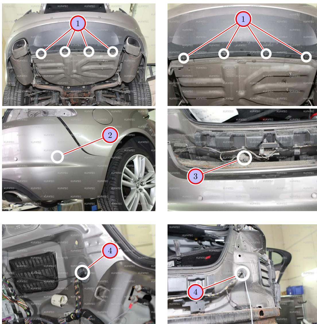
Figure 7: Removing bumper and cable routing
